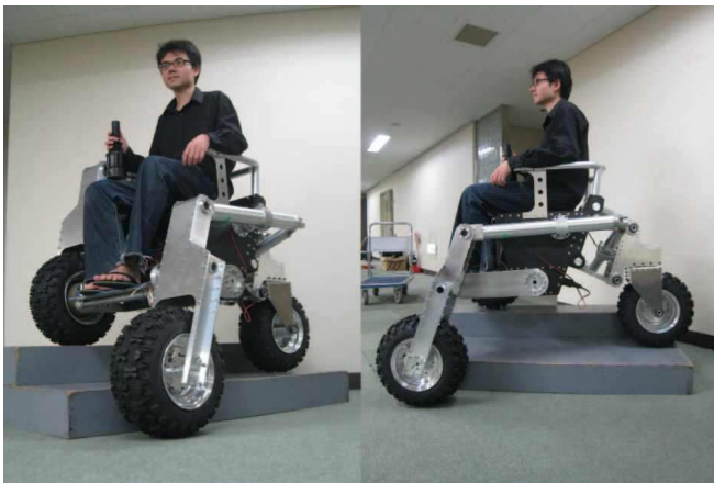
Fig. 1. Proposed three-wheeled body-stabilizing vehicle.
