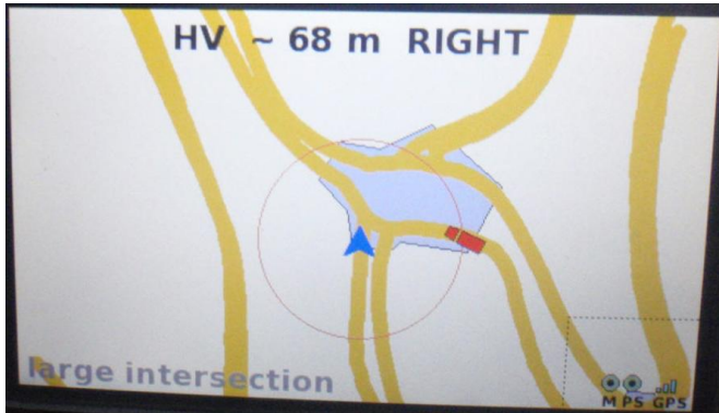
Fig. 2. Photograph of the operator interface module of a safety system. The module is fitted inside the cabin of a haul truck and provides the driver with situation awareness capabilities. Roads are depicted as thick yellow lines and a large intersection is represented as a light blue polygon. The blue arrow denotes the vehicle where the module is fitted and the red box represents a haul truck. Both vehicles are entering an intersection area. In this situation, knowing the set of possible paths for the vehicles is more important for the driver than the actual road map.
