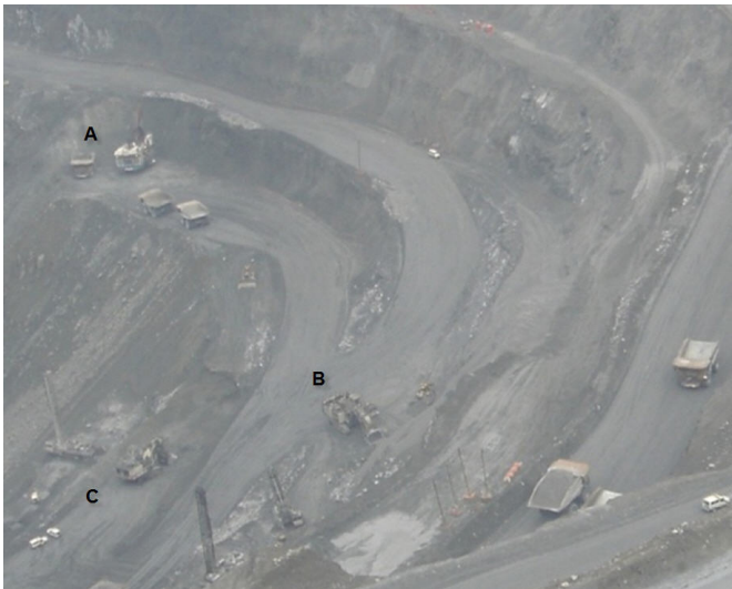
Fig. 1. Snapshot of the operation of a large opencast mine. Loading and drilling areas are marked with letters. See text for details.
