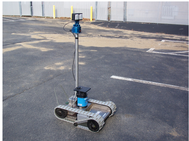
Fig. 1. Daredevil PackBot equipped with a RaDeKL UWB radar on a pan/tilt mount and a SICK LD OEM LIDAR.
