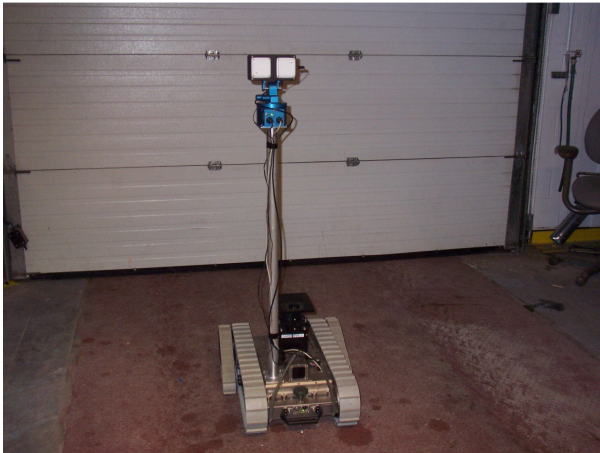
Fig. 5. Daredevil PackBot in fog-free indoor test area
