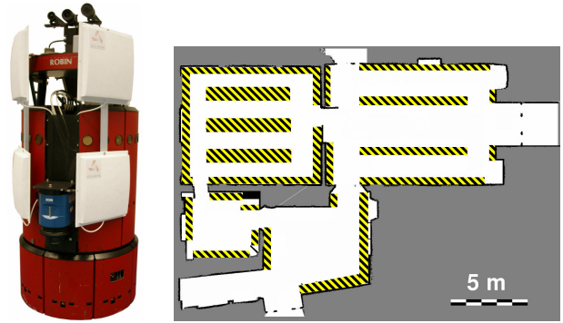
Fig. 2. Left: The mobile robot (RWI B21) used for the experiments, with its UHF RFID antennas (white), spanning an angle of approx. 90^\circ . Right: One of the environments in which we conducted the experiments. Approx. 400 RFID tags had been placed in the hatched areas. The second test area is very similar in size and shape.
