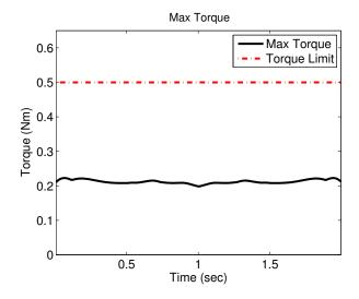
Fig. 7. Maximum joint torque during four-fingered simulations described in Section IV-B.1.
