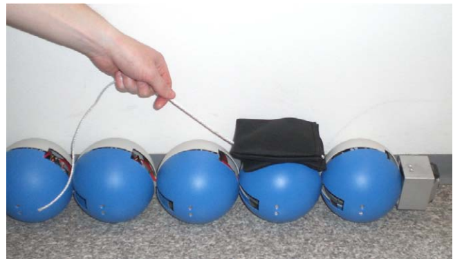
Fig. 17. The setup of the experiment conducted in order to test the contact force measurement system.
