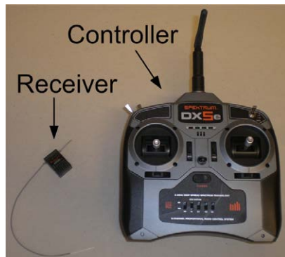
Fig. 16. The remote controller and the receiver used for controlling the snake robot.
