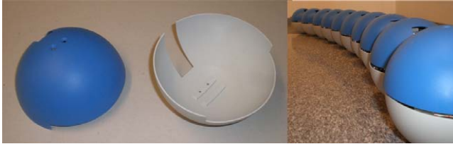
Fig. 6. Left: The upper and lower hemispherical shell of a joint module. Right: The smooth gliding surface along the snake robot.
