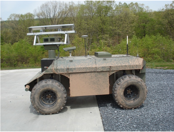
Fig. 2. The eXperimental Unmanned Vehicle (XUV) on a gravel and asphalt (pavement) transition
