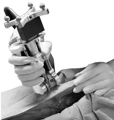
Fig. 1. Wheeled Robot Testing on Swine Skull
