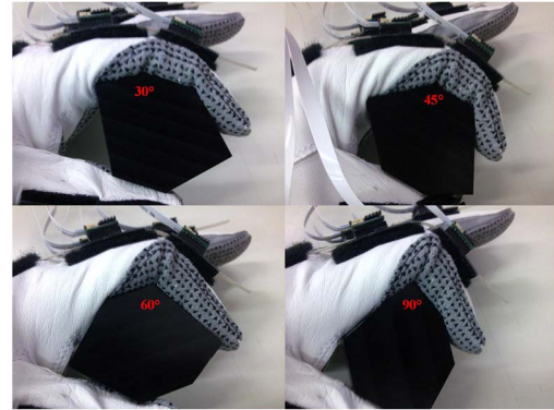
Fig. 9. Calibrate Index Finger's PIP joint using Calibration Block.
