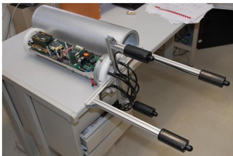
Fig. 4. Prototype system under development: acoustic array and core processing systems
