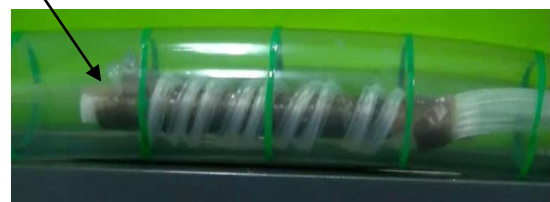
Fig.13 Transportation experiment using two tube actuators winding around dummy endoscope
