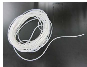
Fig. 6 Developed tube actuator whose cross section is Fig.5; by extrusion molding method, rubber tube can be achieved over 100m with maintaining same cross section shape.
