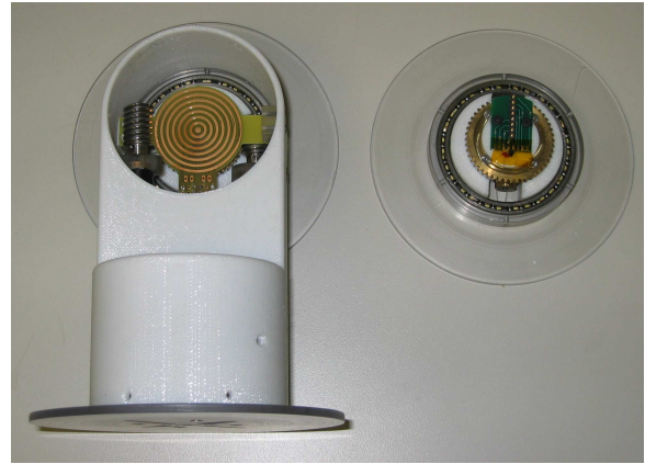
Fig. 4. Module shown with the center wheel removed to show slip ring.
