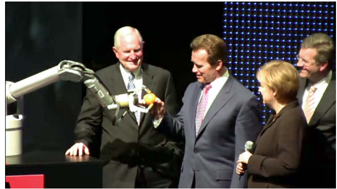
Fig. 10. Governor Schwarzenegger receiving orange from the robot. The robot decides when to release the object based on co-manipulation detection.
