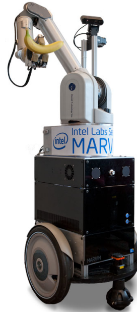
Fig. 1. Photograph of mobile manipulation platform MARVIN, with Electric Field Pretouch-enabled hand. The system includes a Barrett Hand, WAM arm, and Segway base. Each fingertip contains one of our custom electric field sensing boards and 4 sensing electrodes. Another EF sensing board with one transmit electrode is built into the palm, which serves as a hub for aggregating sensor data from the fingertips. The palm also contains a camera, which was not used in the experiments reported in this paper.
