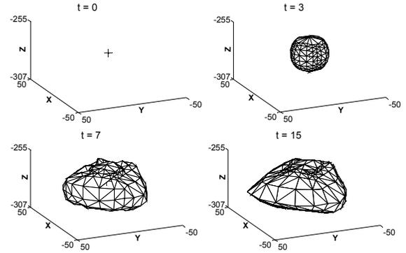
Fig. 7. 3D workspace boundary generation using MPSO ( $[\Phi, \theta, \psi]^T = [0, 0, 0]^T$ ). The MPSO searches from the start point  $c = [0, 0, -270]^T$  denoted by the cross sign. The surface boundary is shown as tessellated from the positions of particles.
