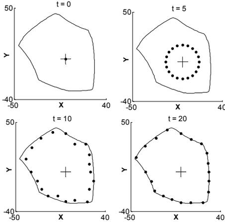
Fig. 5. 2D workspace boundary generation using MPSO ( $Z = -270$  mm and  $[\Phi, \theta, \psi]^T = [0, 0, 0]^T$ ). The MPSO searches from the start point  $c = [0, 0]^T$  denoted by the cross sign.
