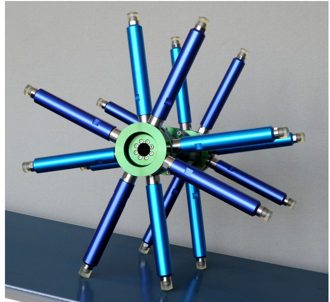
Fig. 1. Spoke-like passive-dynamic walker that consists of two identical crossed frames
