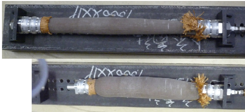
Fig. 2: Overview of the artificial muscle
