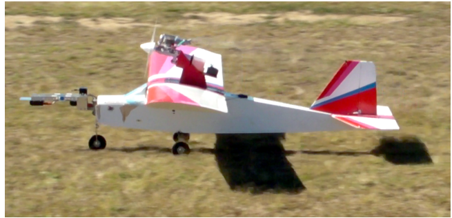
Fig. 1. Implementation of the stereo vision system shown mounted on the test aircraft. The aircraft is a Super Frontier Senior-46 (wingspan 2040mm), modified so that the engine and propeller assembly is mounted above the wing.
