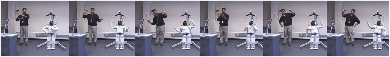
Fig. 8. Snapshots of ASIMO replicating the motion of a human demonstrator in real time.
