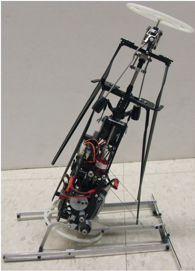
Fig. 3. A prototype of the revised design midway through transformation. The upper rotor is retained close to the robot's body as it tips down, keeping the lower rotor folded as well.
