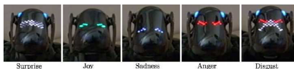
Fig. 7. The figure illustrates the LEDs' configuration for each universal expression.
