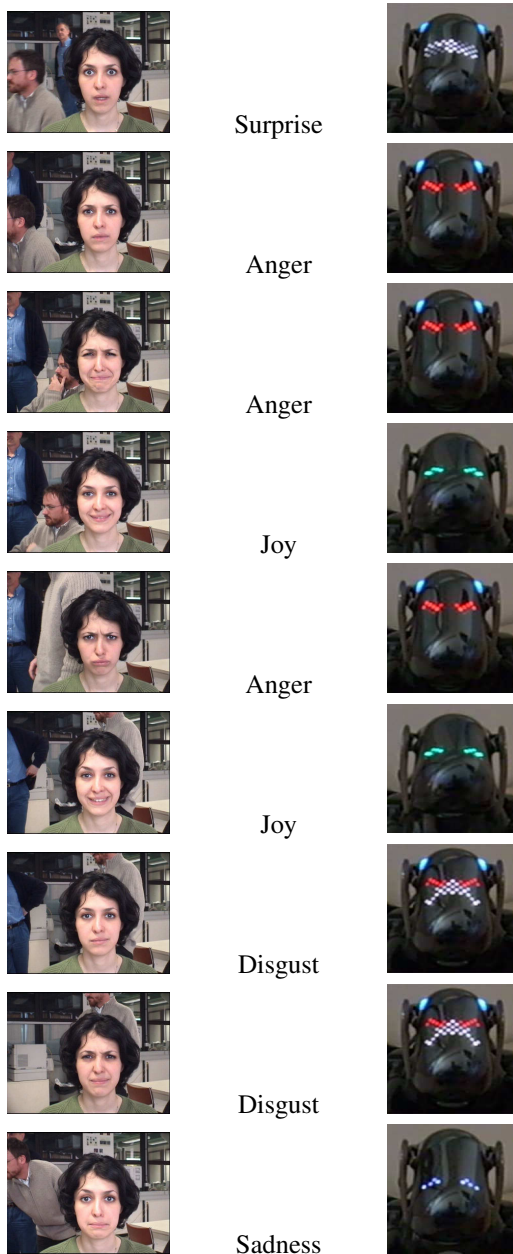
Fig. 8. Person's facial expressions are shown in correspondence with the robot's response.
