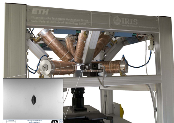
Fig. 1. The OctoMag prototype contains eight 210-mm-long by 62-mm-diameter electromagnets. The gap between two opposing electromagnets on the lower set is 130 mm. The inset is the side-camera view, and shows a 2-mm-long microrobot of the type described in [5].
