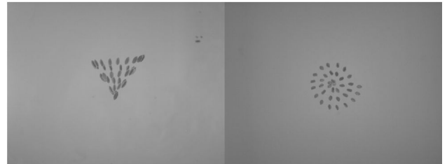
Fig. 6. Demonstration of automated pose control. Both time-lapse image sequences show a 500- \mu\text{m} -long microrobot following a spiral trajectory keeping its orientation constantly pointing at the vertex of the spiral. The left image shows a side view, and the right image shows a top view. Average trajectory-completion time: 33.4 s.
