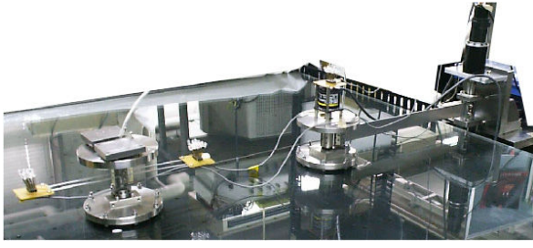
Fig. 1. Experimental setup of manipulator with two lightweight links and a free joint
