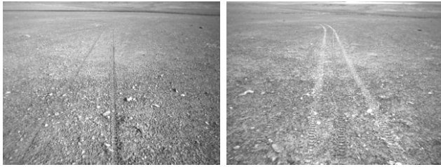
Fig. 12. Images from the teach (left) and repeat (right) passes of a route on Devon Island. The rover was unable to localize for 50 meters even though it was clearly on the path.
