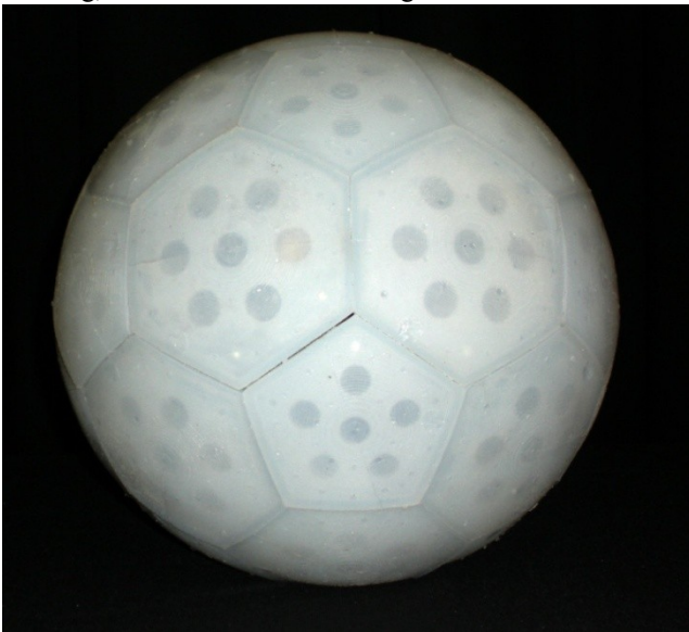
Fig. 8. The assembled spherical robot.
