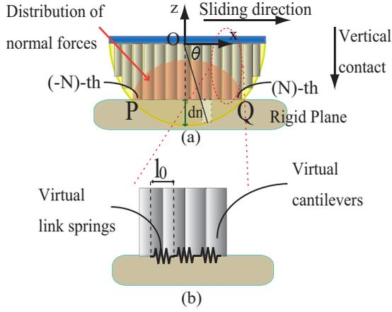
Fig. 2. Proposed model of a soft fingertip comprised of virtual elastic cantilevers.
