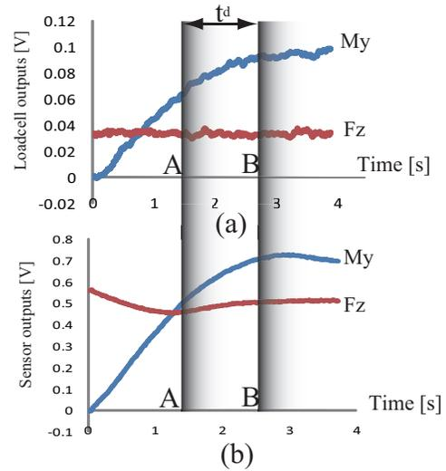
Fig. 8. Signals of normal forces ( $F_z$ ) and tangential moments ( $M_y$ ) from: (a) Load cell. (b) Sensor.
