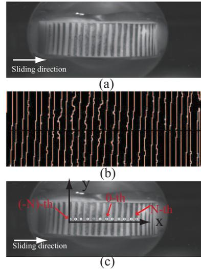
Fig. 10. Images for processing: (a) Grayscale image. (b) Binary image with extracted edges. (c) Image with tracked points.
