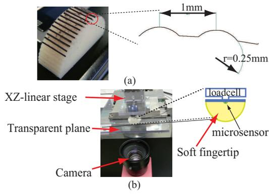
Fig. 7. Experiment set-up a) Semi-cylindrical soft fingertip and the distributed ridges on the surface. b) Entire view of the experimental apparatus.
