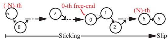
Fig. 6. Orders of movement of virtual cantilevers' free-ends during the stick-to-slip transition.
