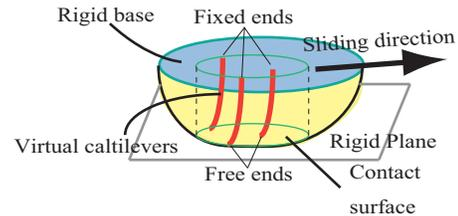
Fig. 1. Proposed model of a soft fingertip comprising of virtual elastic cantilevers. (a) Distribution of normal forces when the fingertip is pushed. (b) Virtual cantilevers and linkage springs are introduced.
