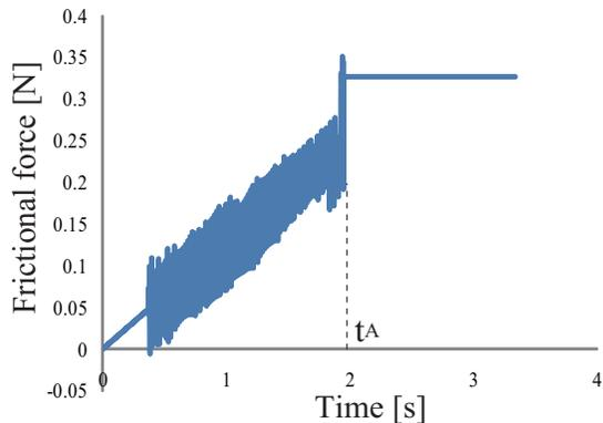
Fig. 4. Simulation results: Response of frictional force acting on the contact surface during stick-to-slip transition.
