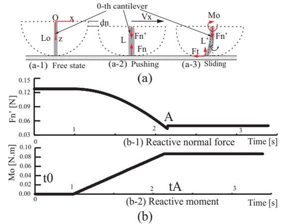
Fig. 9. Model of force/moment acting on the fixed-end of the 0-th cantilever: (a) Contact States of the cantilever. (b) Graphs of force and moment acting on the cantilever.
