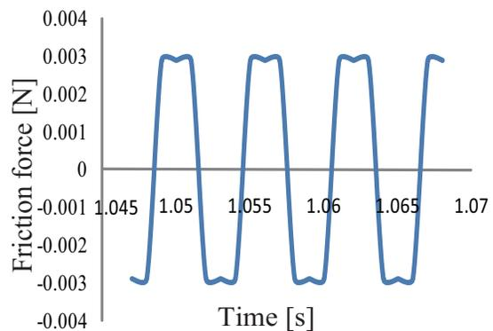
Fig. 5. Simulation results: Magnification of response of frictional force acting on an arbitrary cantilever's free-end.
