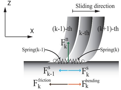
Fig. 3. Forces acting on  $k$  cantilever.
