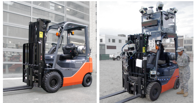
Fig. 1. (left) The platform is a stock 2700kg Toyota lift truck that we developed into (right) an autonomous vehicle that operates outdoors in proximity to people; a military supervisor stands nearby. A safety driver may sit in the cabin, but does not touch the controls.
