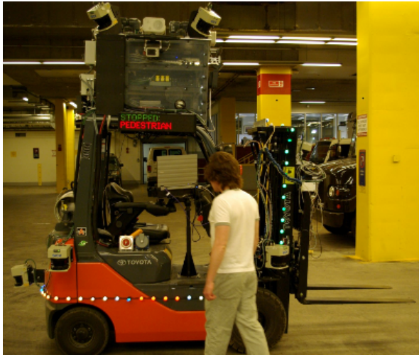
Fig. 5. An approaching pedestrian causes the robot to pause. Lights skirting the robot indicate distance to obstacles (green:far to red:close). Verbal annunciators and signage indicate the induced pause.
