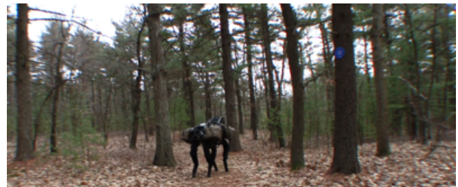
Fig. 8: BigDog during autonomy distance testing.
