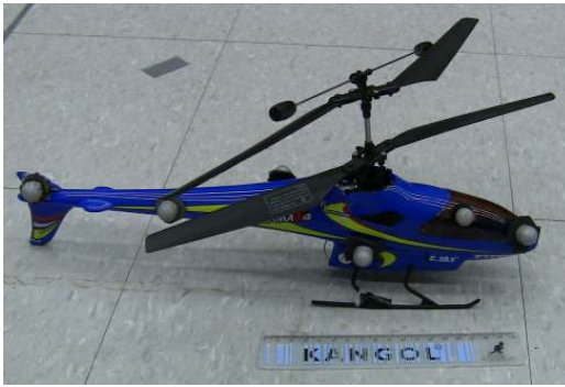
Fig. 1. Esky LAMA V4 Helicopter. An Esky LAMA V4 helicopter used in the ARCLab. Note the attached reflective markers tracked by the Vicon camera system.
