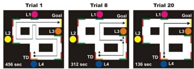
Fig. 7. Routes followed by one of the robots in locating the goal during three training trials from a fixed departure location (TD) being oriented north in the cyclic maze. Illustrated trials were taken from beginning (Trial 1), middle (Trial 8), and end (Trial 20) of the learning process. The line inside each maze represents the route followed by the robot. The small arrow placed at location TD indicates the robot orientation. The average latency of arrival to the target in those three training trials is shown below each maze.
