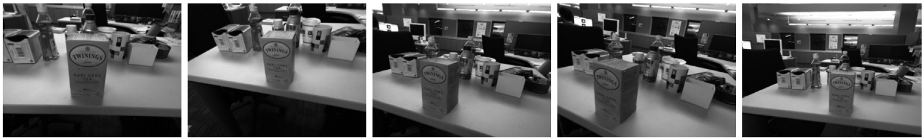
Fig. 2: Example keyframes of the teabox object. The keyframes are saved during offline analysis and later utilized in the GPE.
