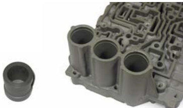
Fig. 4. Transmission valve body (left) and spool insert (right) to be assembled by the robotic manipulator.
