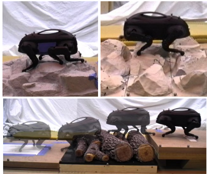
Fig. 1. Boston Dynamics Inc. LittleDog quadruped robot, shown crossing several types of rough terrain.
