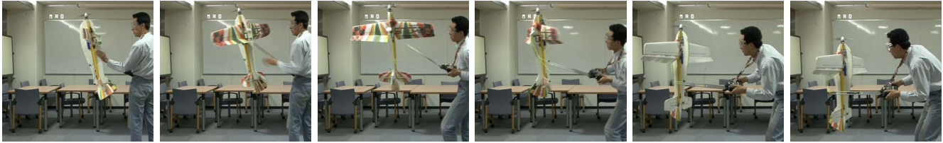
Fig. 11. Resolved tilt-twist angle control experiment. Since large aileron angle caused drag force, the UAV lost altitude slightly. However, the UAV could continue hovering stably.
