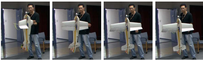
Fig. 14. Human inflicted rotational disturbance while hovering with resolved tilt-twist angle control, but the UAV continued hovering stably.
