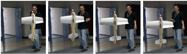
Fig. 15. Human inflicted translational disturbance while hovering with resolved tilt-twist angle control, but the UAV continued hovering stably.
