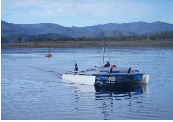
Fig. 3. The ASV is integrated with an array of 50 floating sensor network nodes (orange buoy behind the ASV) for communication and event detection. The ASV is capable of detecting a node and maintaining a minimal stand off distance to allow in situ calibration of the nodes sensors.
