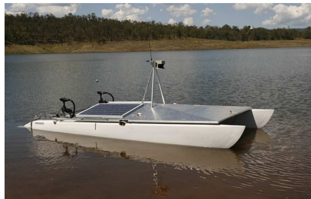
Fig. 1. The solar-powered Lake Wivenhoe ASV.
