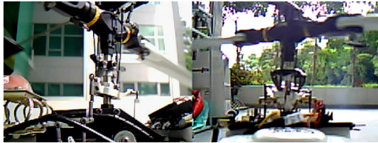
Fig. 9. In the experiments, the fully instrumented hingeless helicopter (JR Voyager GSR) is commanded to pitch and roll on the ground. The onboard computer records the inputs to the rotor from servomechanisms, and the IMU measures the inclination information.
