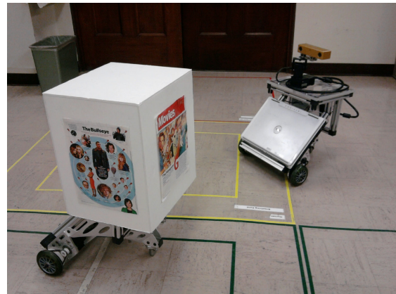
Fig. 1. The setup of our experiment is shown above where the mobile agent is equipped with a stereo-camera head mounted to a pan-tilt unit. The object to be identified is also mobile with the mobile component also a two-wheeled nonholonomic robot controlled by an external operator.
