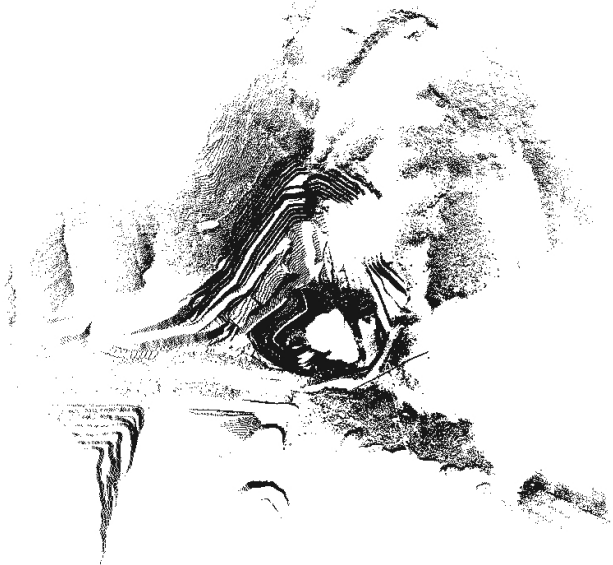
Fig. 4. Laser data 1: RIEGL Laser scanner based dense scan taken at Mt. Tom Price. It consists of over 850,000 points spread over 2146.6 m x 2302.1 m x 464.3 m
