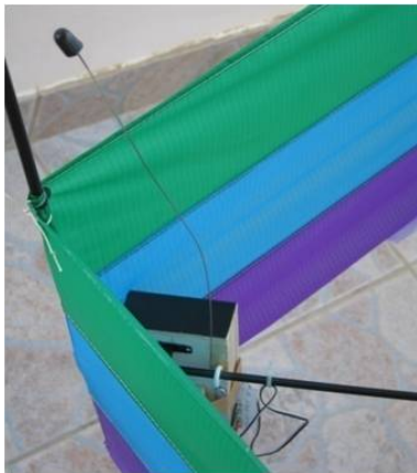
Fig. 6. The wireless control receiver suspended on one of the lower struts.
