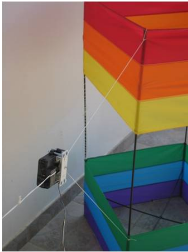
Fig. 5. The proposed bridle adjustment actuation unit.
