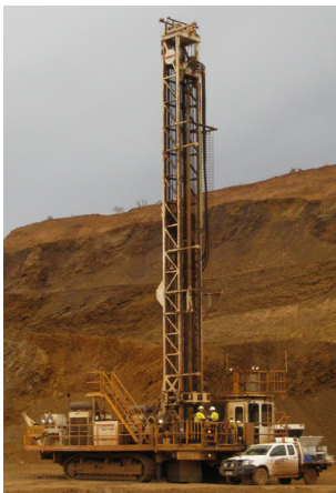
Fig. 1. The autonomous blast hole drill rig at rest on a drill bench of an open-pit mine (the 4x4 truck illustrates the large scale).
