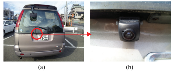
Fig. 7 (a) The back side of the vehicle used in our experiment. (b) The used rear view camera.
