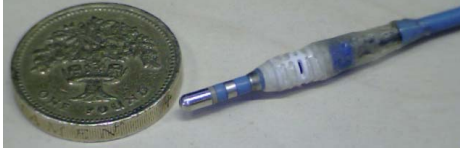
Fig. 2. Photograph of the fibre-optic sensor prototype integrated with a 7 Fr catheter. A one GB-pound coin is shown for comparison.
