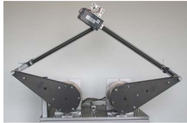
Fig. 1. Planar parallel manipulator FIVEBAR
