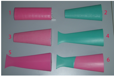
Fig. 4. Compliant prototypes used in the experiments. The prototypes are manufactured using two different silicone materials: i) Elite Double 22 (green) and Elite Double 8 (pink). The elasticity values for E8 and E22 are, respectively, around 450\text{KPa} and 720\text{KPa} .
