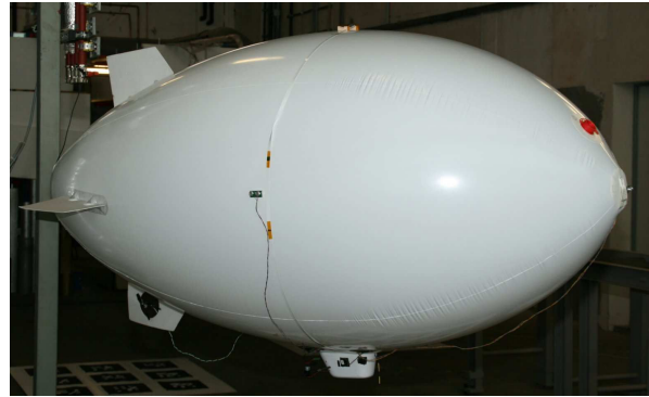
Fig. 1. The robotic indoor blimp [19] used throughout this paper. It is actuated by two main propellers that pivot together and a third laterally mounted rear propeller. Four small, lightweight wide-angle sonar sensors provide distance measurements to the environment.
