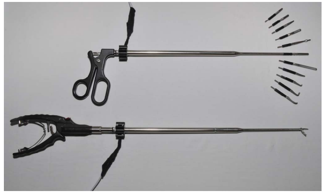
Fig. 1. Prototypes showing the different types of handles and tips that can be used.
