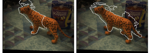
Fig. 9. Segmentation results without color measurements. The images show the 1st and 7th frames of a sequence.
