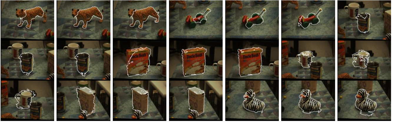
Fig. 2. Segmentation results for every fourth frame of a sequence generated by the attention system. Segmentation is re-initiated after each saccade.
