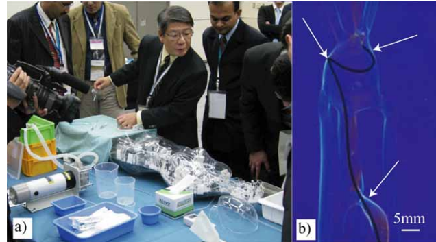
Fig. 1: a) Endovascular Surgery Simulator. b) Birefringence consequence of stress applied to the vasculature model by a guide wire.
