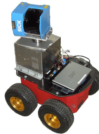
Fig. 1. Our robot platform: Pioneer P3-AT, which carries a SICK LMS laser range scanner mounted vertically on a rotating disk. Image courtesy of Timo Röhling.
