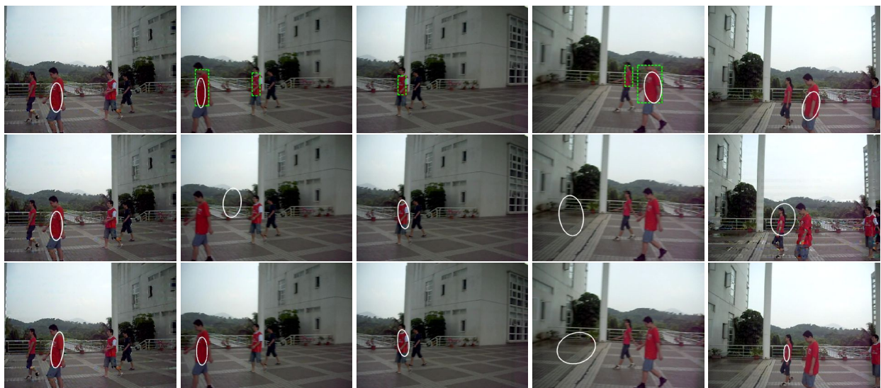
Fig. 11. The comparison of tracking results when camera has strong jerks and the frame content changes dramatically.( frame: # 118, #120, #122, #125, #127) 1 st row: our model. 2 nd : mean-shift 3 rd : improved mean-shift for motion blur.
