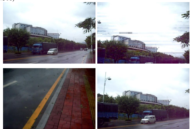
b) Strong jerk. Camera is bumped strongly and recovers at once. The frame content changes dramatically. (Frame #40, #41, #43, #46)
