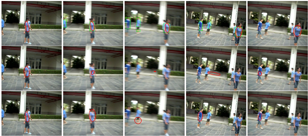
Fig.10. The comparison of tracking results when camera has fast motion and it cause motion blur. (Frame: # 715, #720, #722, #725, #726) 1 st row: our model. 2 nd : mean-shift 3 rd : improved mean-shift for motion blur.
