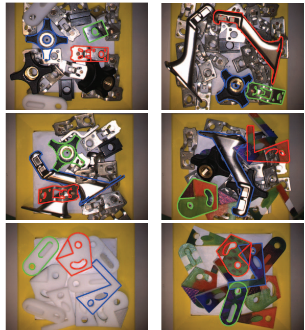
Fig. 11: Performance on real examples. The system detected and accurately estimated the pose for specular as well as textureless objects. Shown in these images are the top detector outputs for three different objects overlaid on top of the original images.
